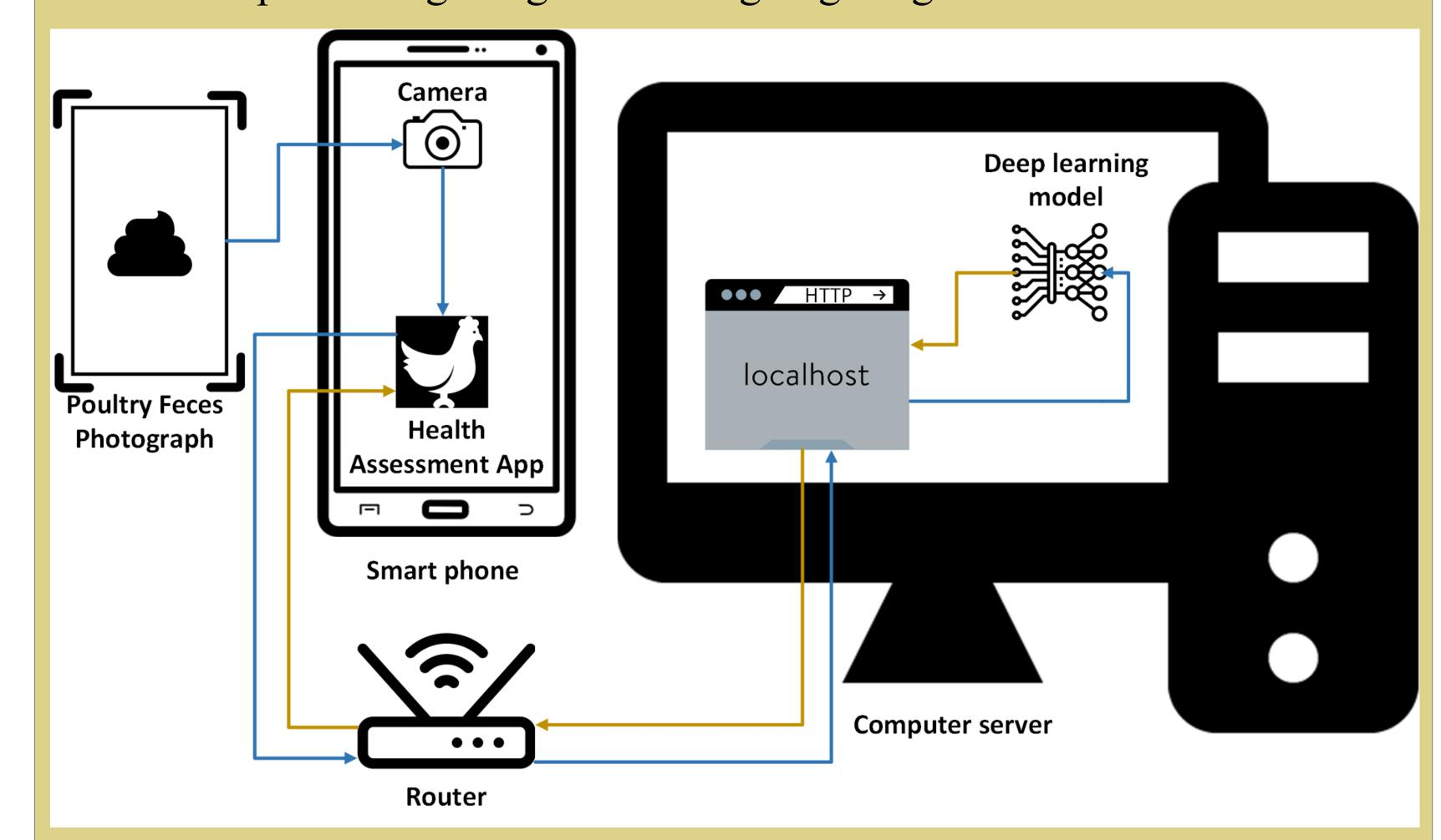
Fig 2. Overall framework of the poultry health assessment system. Blue lines indicate the pathways of transferring a raw image, and yellow lines indicate the pathways of transferring a processed image.
